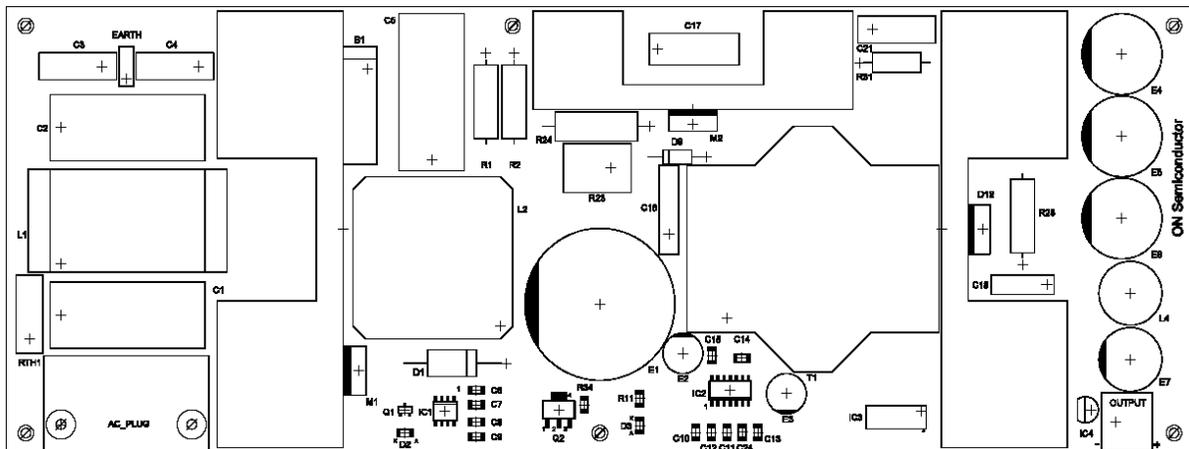
Figure 12. Top View of Component Side
