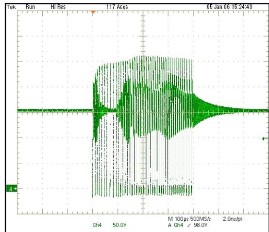
Figure 9. Detail of a Skip Burst
