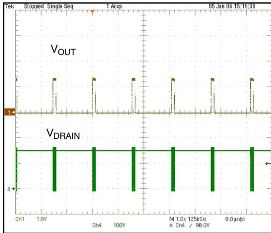
Figure 6. Short-circuit Burst Mode
