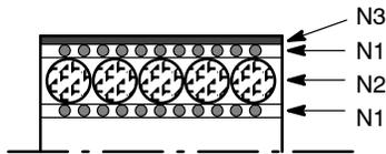
N1 — 11 turns of multiwire 20 x  $\phi 0,2$  mm 3 kV isolation
