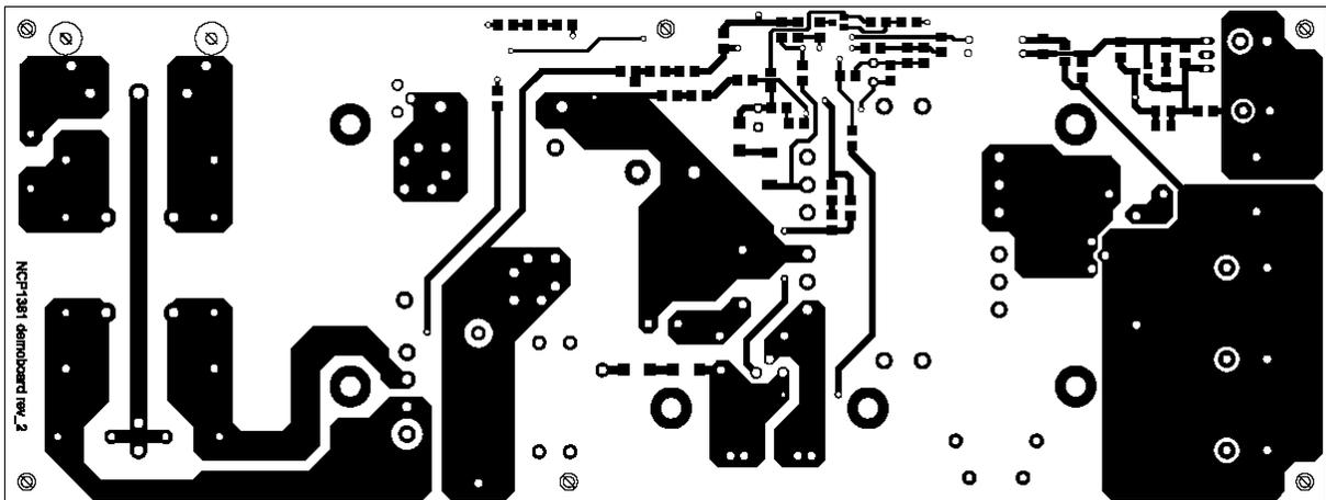
Figure 10. Solder Side (bottom view)
