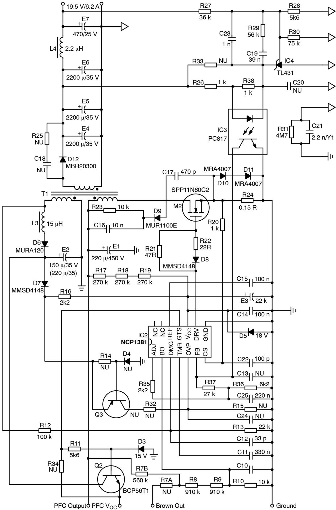
Figure 2. Valley Switching Converter
