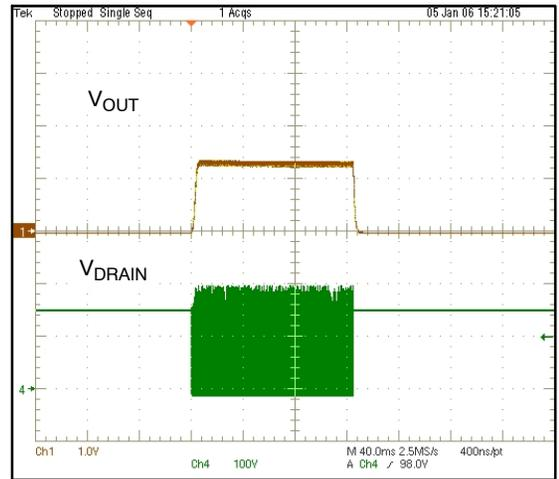
Figure 7. Detail of a Short-circuit Burst
