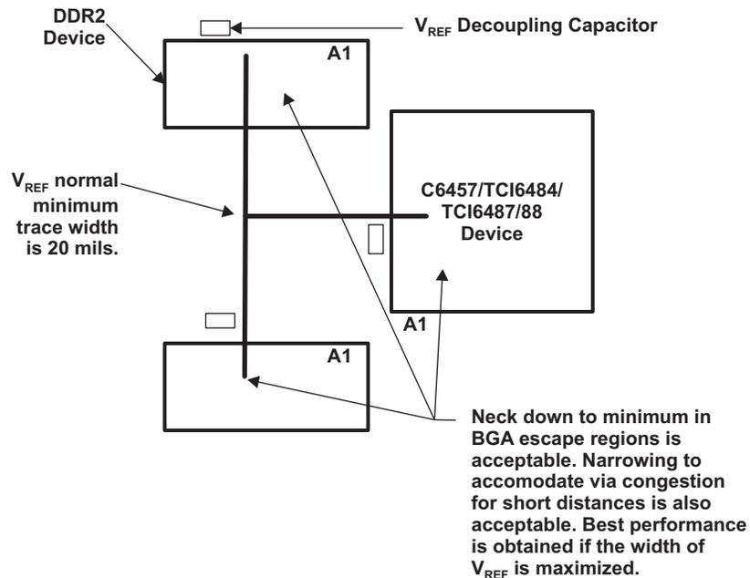
Figure 3.  $V_{REF}$  Routing
