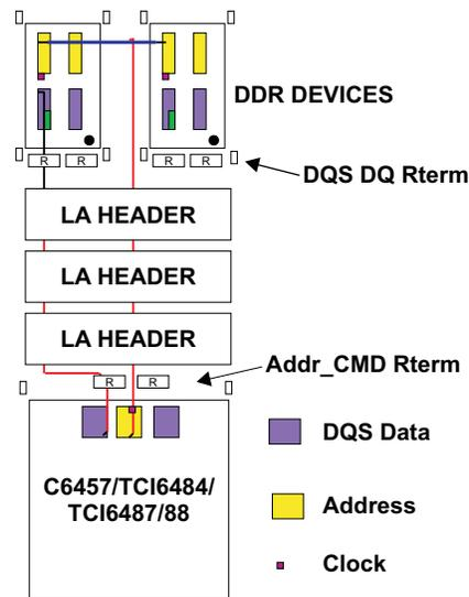
LA Header refers to the logic analyzer header. This is typically not present, nor recommended, in production applications as it may impact memory performance.
