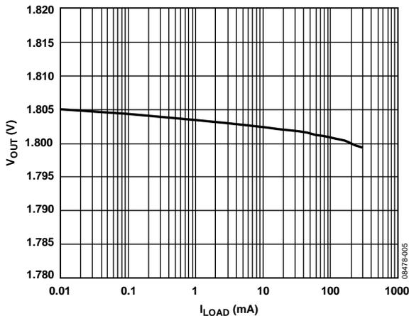
Figure 5. Output Voltage,  $V_{OUT}$  vs. Load Current,  $I_{LOAD}$  at  $V_{IN} = 2.3 V$ ,  $V_{OUT} = 1.8 V$ ,  $T_A = 25^\circ C$
