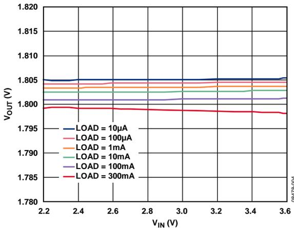
Figure 4. Output Voltage ( $V_{OUT}$ ) vs. Input Voltage ( $V_{IN}$ ) at  $T_A = 25^\circ C$
