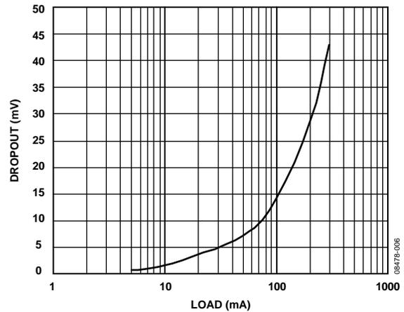
Figure 6. Dropout Voltage vs. Load Currents ( $I_{LOAD}$ )
