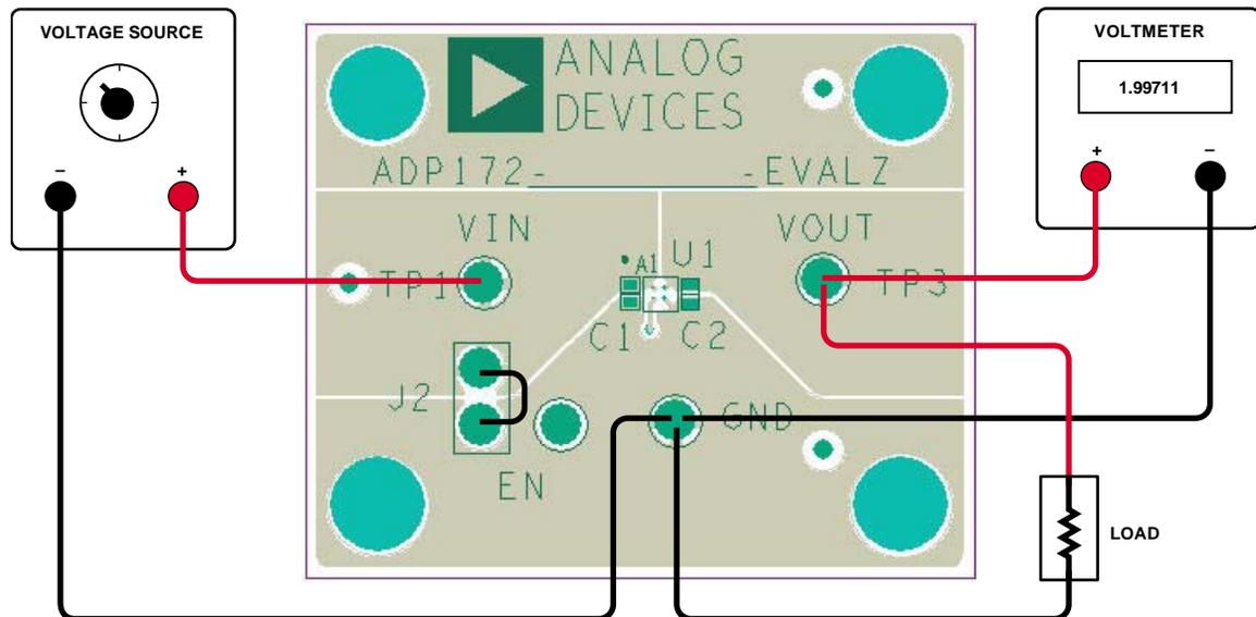
Figure 3. Output Voltage Measurement Setup, WLCSP
