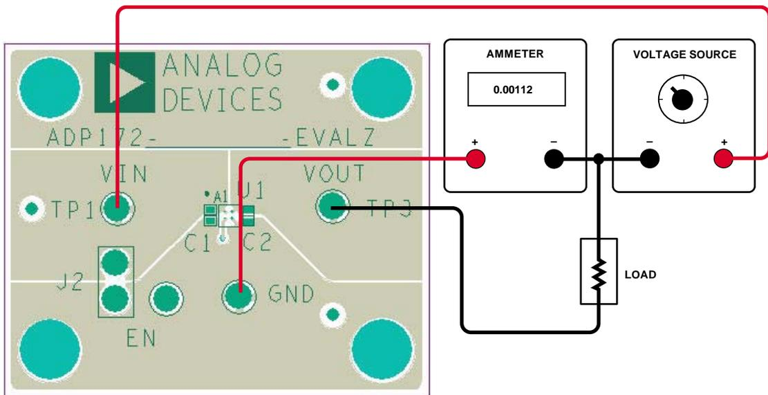
Figure 8. Ground Current Measurement Setup, WLCS
