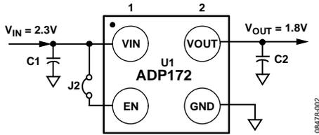
Figure 2. Evaluation Board Schematic, WLCSP
