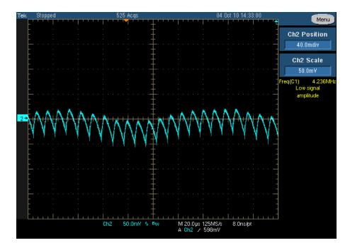
9.6V output ripple voltage in @ 400mA load and no load on 5V.
