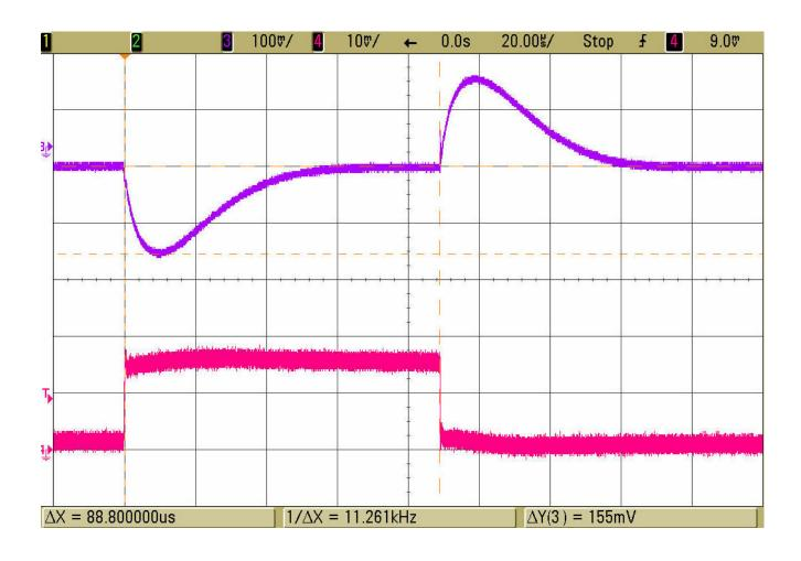
Figure 4. Load Step Response  $V_{IN}$  = 3.3V,  $V_{OUT}$  = 1.8V, 2.5A Load Step (0.5A <-> 3A)
