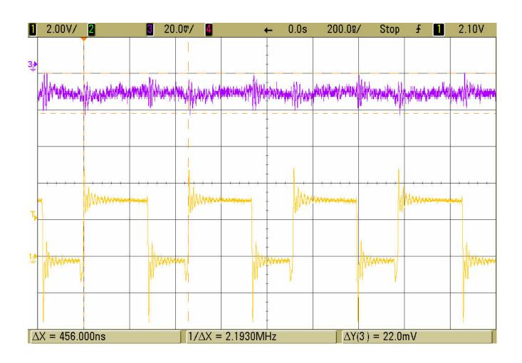
Figure 3. Switch Node & Output Ripple Voltage Waveforms
