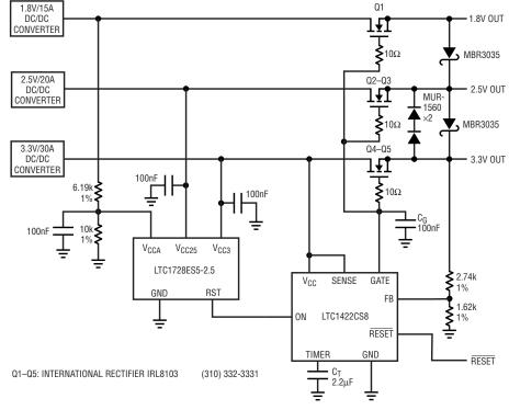
Figure 1. Ramping three supplies
