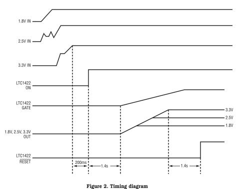
Ramp Three Supplies... continued from page 25 When all supplies rise to within acceptable limits (typically within 7.5% of the nominal output voltage), the LTC1728 waits 200ms and then enables an LTC1422 Hot Swap™ controller. The LTC1422 introduces an additional delay of approximately 1.4 seconds and then ramps the gates of three N-channel MOSFETs, one in series with the output of each supply. Figure 2 shows the relative timing of various waveforms during start-up.
