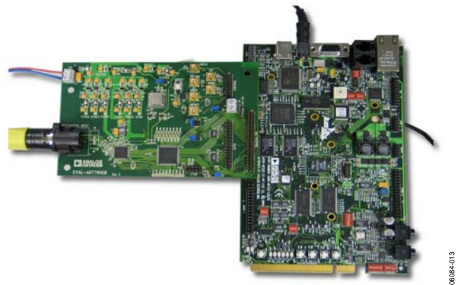
Figure 13. Powered Up AD7764/AD7765 Evaluation Kit
