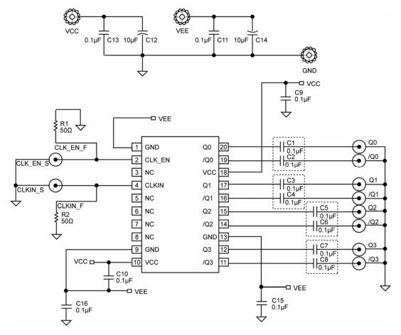
Note: R1 and R2 terminate trace at SMA pad.
