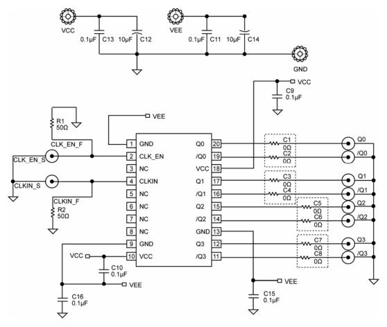
Note: R1 and R2 terminate trace at SMA pad.
