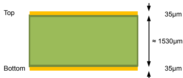
Figure 4-6. PCB layer stack.
