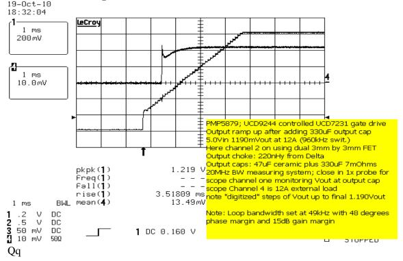
Output transistions when Most significant Bit (MSB) of VID switched: This bit switches Vout by 240mV:
