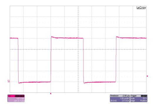
The photo below is of the N-ch FET drain waveform (TP7). The input voltage is 200Vand the output is loaded to 0.05A. (100V/DIV, 1uS/DIV)
