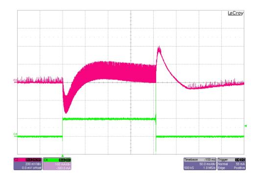
The photo below shows the 200V output voltage (AC coupled) when the load current is pulsed between 0A and 0.2A. Rising edge only. Vin = 200Vdc. (200mV/DIV, 100mA/DIV, 50mS/DIV)
