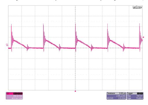
The 200V output ripple voltage is shown in the figure below. The image was taken with the output loaded to 0.1A and the input voltage set to 200Vdc. (200mV/DIV, 2uS/DIV)
