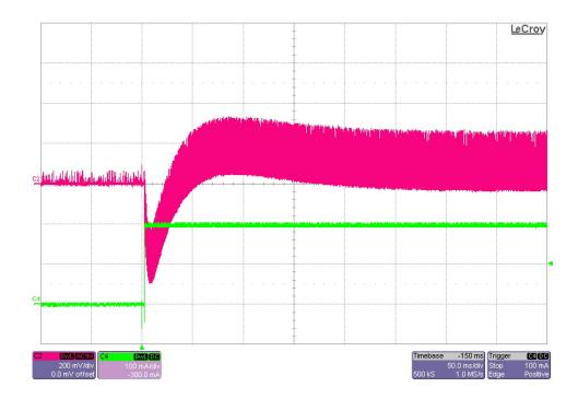
The photo below shows the 200V output voltage (AC coupled) when the load current is pulsed between 0A and 0.2A. Falling edge only. Vin = 200Vdc. (200mV/DIV, 100mA/DIV, 50mS/DIV)
