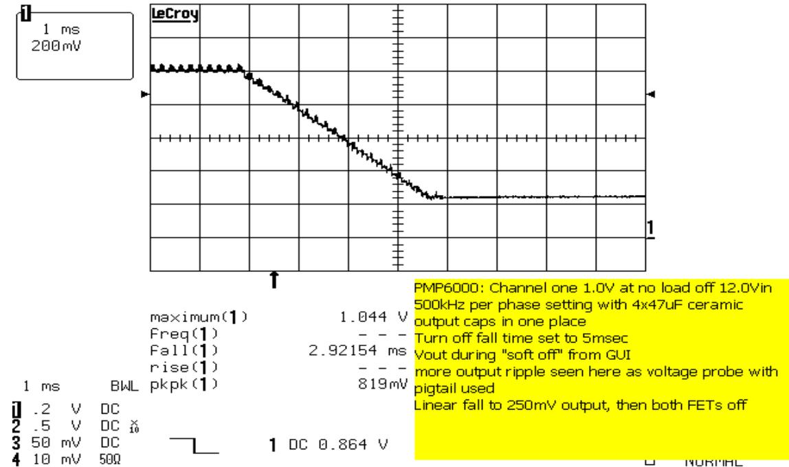
Output ripple with close in 1x probe:
