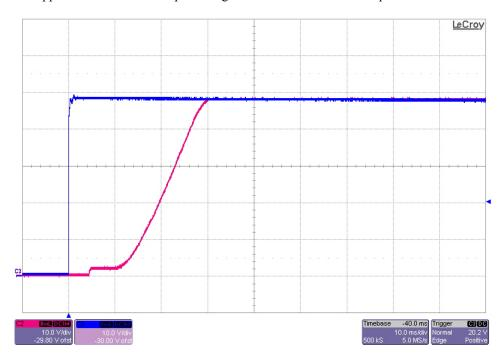
The output startup waveform is shown in the figure below after the application of Vin. The input voltage was set to 48V and the output was loaded to 0.7A.
