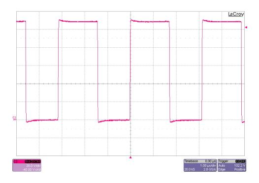
The figure below shows the switch node waveform (TP4) for Vin = 60V and Iout = 0.09A. (20V/DIV, 1uS/DIV)
