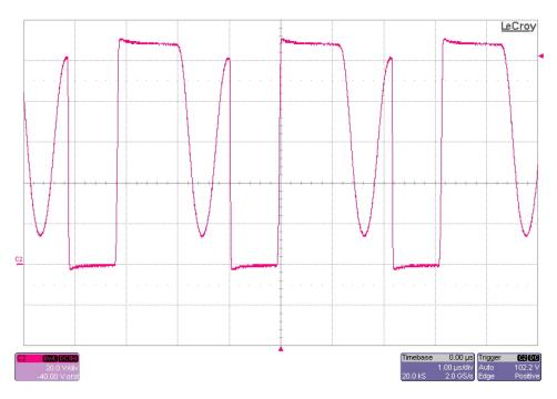
The figure below shows the switch node waveform (TP4) for Vin = 40V and Iout = 0.7A. (20V/DIV, 1uS/DIV)
