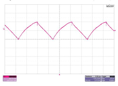
The 48V output ripple voltage is shown in the figure below. The image was taken with a 0.7A load and Vin set to 40V
