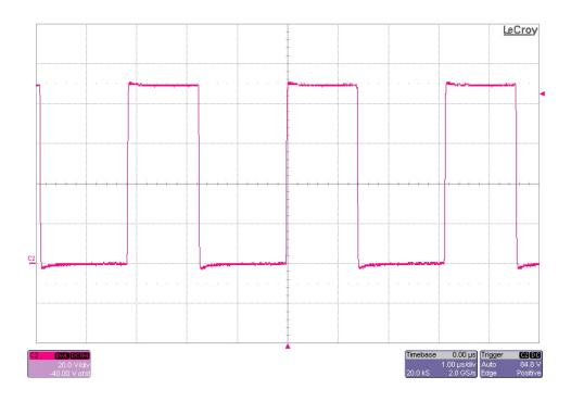
The figure below shows the switch node waveform (TP4) for Vin = 40V and Iout = 0.09A. (20V/DIV, 1uS/DIV)
