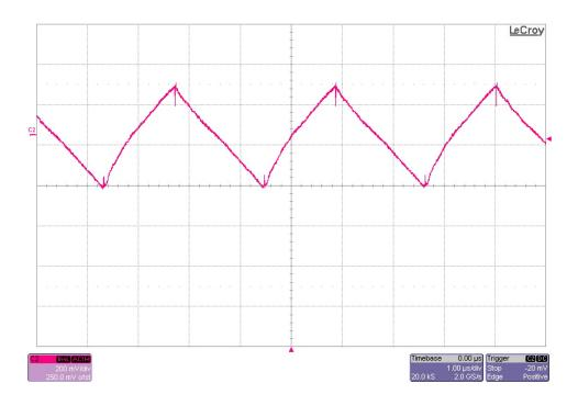
The 48V output ripple voltage is shown in the figure below. The image was taken with a 0.3A load and Vin set to 48V
