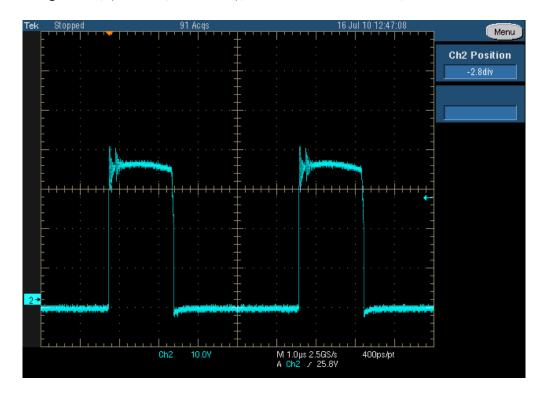
Channel 2: "Q9 Vds", (10V/div, 1usec/div), no bandwidth reduction, @ 36Vin
