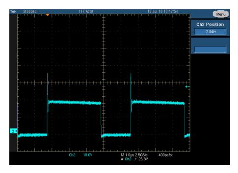
Channel 2: "Q11 Vds", (20V/div, 1usec/div), no bandwidth reduction, @ 36Vin
