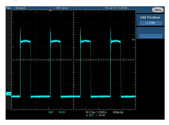
Channel 2: "Q6 Vds", (10V/div, 2usec/div), no bandwidth reduction, @ 36Vin
