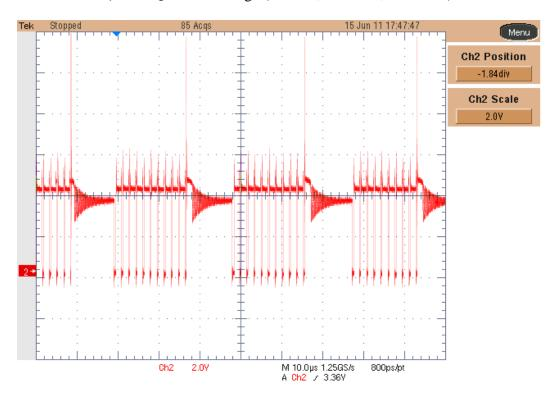
Output current = 2.4A, Ch2: Q2 drain voltage (2 V/div, 400ns/div, No BWL)
