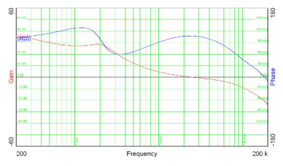
The next figure shows the bode plot with a 24V input , 12V output at 180mA (discontinuous conduction mode).
