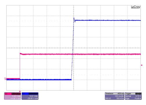
The photo below shows the 56V output voltage startup waveforms after the application of 48Vdc in. The output was loaded to 0A. (Vin is 10V/DIV, Vout is 10V/DIV, 100mS/DIV)
