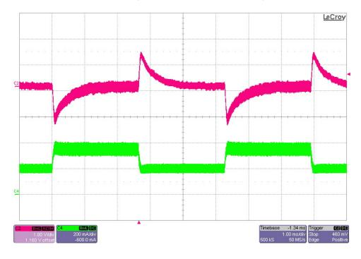
The photo below shows the response of the 56V output voltage (ac coupled) to the load current stepping between 0.20A and 0.35A. Vin = 24Vdc. (1V/DIV, 200mA/DIV, 1mS/DIV)
