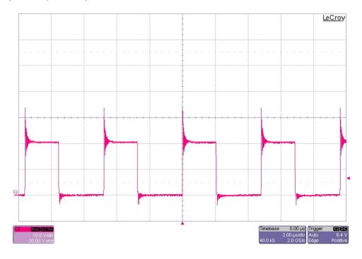
The photos below show the FET drain voltage at TP3. The input voltage is 57V and the output is loaded to 0.35A. (20V/DIV, 2uS/DIV)
