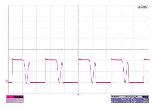
The photos below show the FET drain voltage at TP3. The input voltage is 57V and the output is loaded to 0.05A. (20V/DIV, 2uS/DIV)
