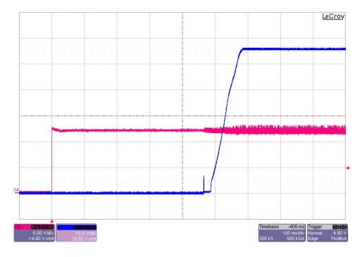
The photo below shows the 56V output voltage startup waveforms after the application of 48Vdc in. The output was loaded to 0.35A. (Vin is 10V/DIV, Vout is 10V/DIV, 100mS/DIV)
