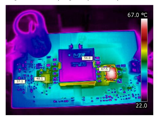
A thermal image is shown below when operating at 12V input and 0.35A output.
