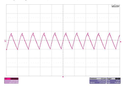
The 56V output ripple voltage is shown in the figure below. The image was taken with the output loaded at 0.35A and the input voltage set to 24Vdc. (200mV/DIV, 5uS/DIV)
