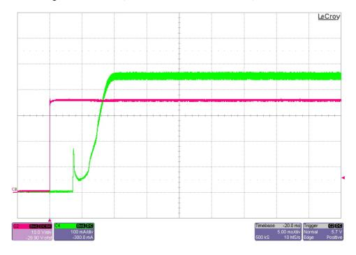
The photo below shows the output current startup waveforms after the application of 48V in. 12 LEDs were used in series and regulated to 0.46A. (10V/DIV, 100mA/DIV, 5mS/DIV)
