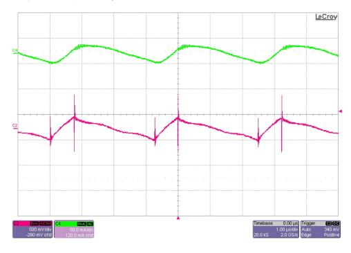
The ac-coupled LED ripple current and voltage (to ground) is shown in the figure below. The image was taken with the output loaded with 12 LEDs and regulated to 0.46A. The input voltage set to 48V. (500mV/DIV, 50mA/DIV, 1uS/DIV)
