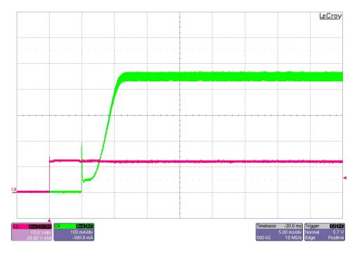
The photo below shows the output current startup waveforms after the application of 24V in. 12 LEDs were used in series and regulated to 0.46A. (10V/DIV, 100mA/DIV, 5mS/DIV)
