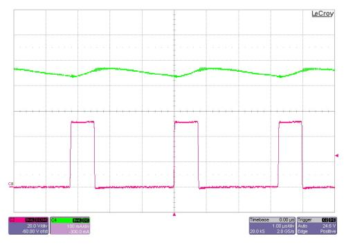
The photo below shows the (Q3) FET switch node and the LED current. The image was taken with an output of 12 LEDs and regulated to 0.46A. The input voltage was set to 24V. (20V/DIV, 100mA/DIV, 1uS/DIV)
