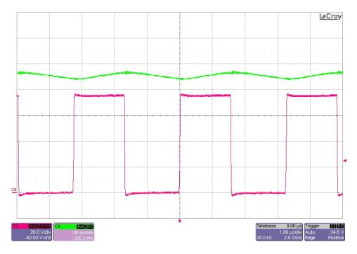
The photo below shows the (Q3) FET switch node and the LED current. The image was taken with an output of 12 LEDs and regulated to 0.46A. The input voltage was set to 48V. (20V/DIV, 100mA/DIV, 1uS/DIV)
