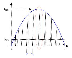
$$I_{\text{IN-AVE}} = \frac{P_{\text{OUT}}}{\eta \times V_{\text{DC-MIN}}} = 550 \text{mA}$$
