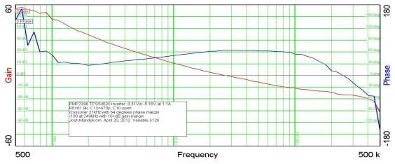
3.3Vin and various loads off -5.16V from 1.1A down to zero A and 3.6V no load:
