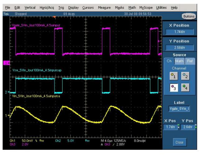
Input voltageSwitch node voltageGate voltage
