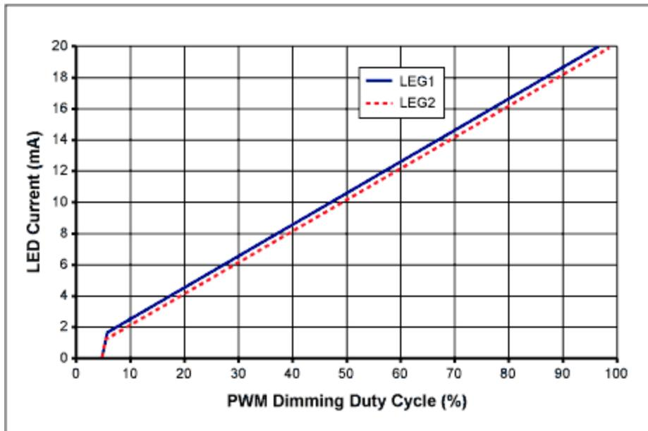
Figure 2. PWM dimming adjusts LED current and controls 1 $\mu$ A shutdown mode. Leg-to-leg current matching is good (better than 5%).
