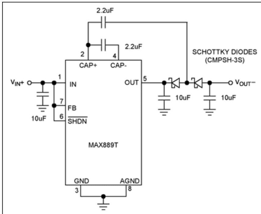
Figure 1. This simple circuit derives -10V from +5V.
