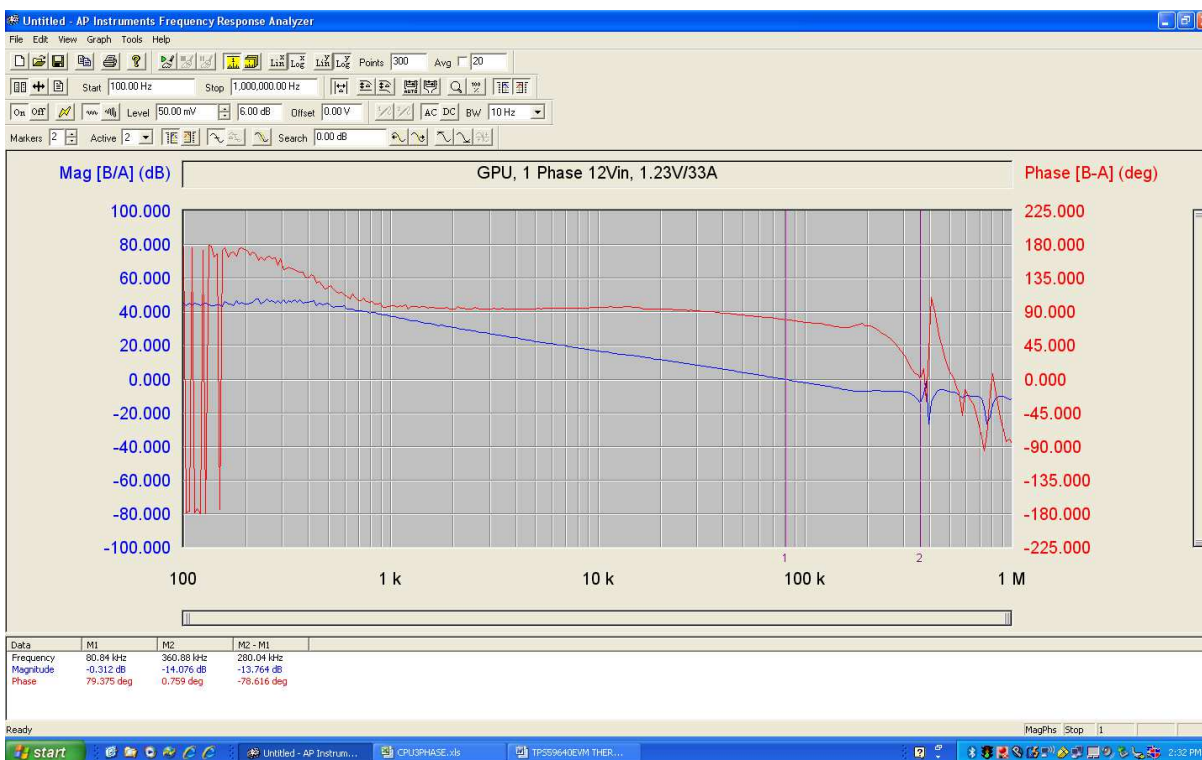
Figure 71. GPU1 Bode Plot at 12Vin, 1.23V/33A
