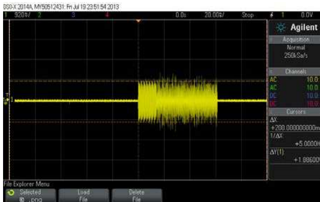
Figure 2-2. Test Results: One Master and Four Slaves
