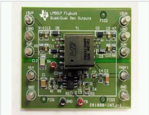
Flybuck Quad Isolated Output Power Supply without Opto-coupler
