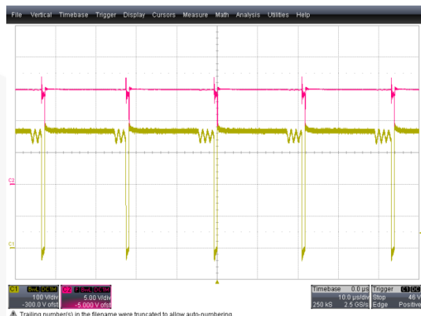
Figure 11. Full-Load Condition, 265 V AC (CH1: V DS (100 V/div), CH2: V CC (5 V/div), Time: 10 μs/div)
