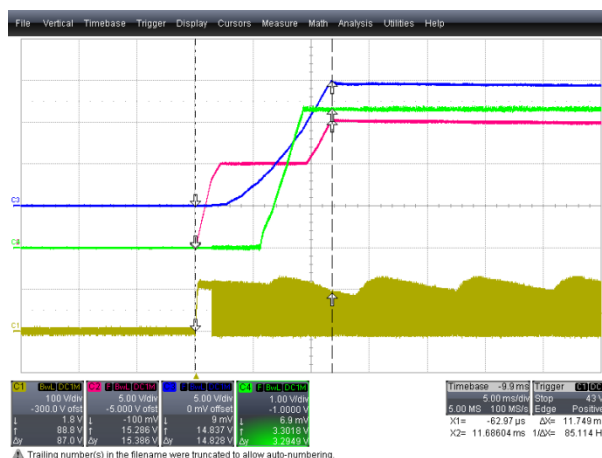
Figure 6. Startup Time=11.7 ms, 85 V AC , Full-Load Condition (CH1: V DS (100 V/div), CH2: V CC (5 V/div), CH3: 15 V OUT (5V/div), CH4: 3.3 V OUT (1 V/div), Time: 5 ms/div)
