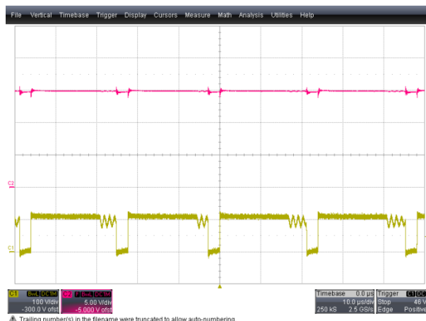
Figure 10. Full-Load Condition, 85 V AC (CH1: V DS (100 V/div), CH2: V CC (5 V/div), Time: 10 μs/div)
