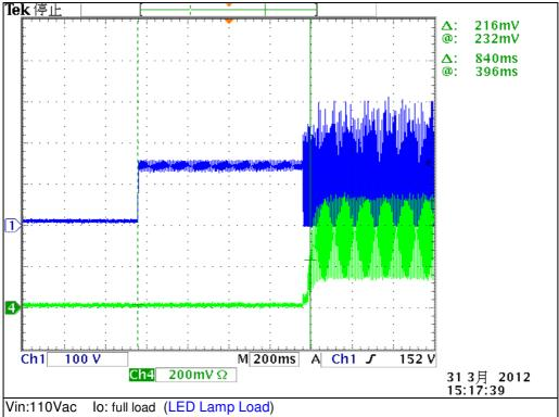
Vin:110Vac Io: full load (LED Lamp Load) Ch1: Vds voltage of MOSFET 100V/div Ch4: LED current 200mA/div
