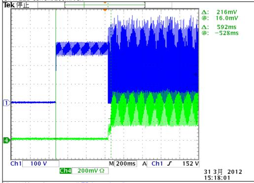
Vin:230Vac Io: full load (LED Lamp Load) Ch1: Vds voltage of MOSFET, 100V/div
