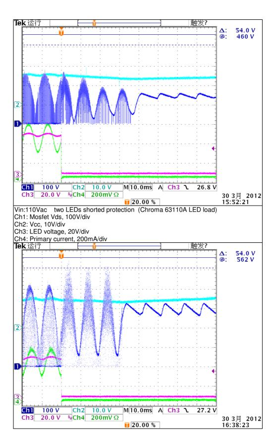
Vin:230Vac two LEDs shorted protection (Chroma 63110A LED load) Ch1: Mosfet Vds, 100V/div
