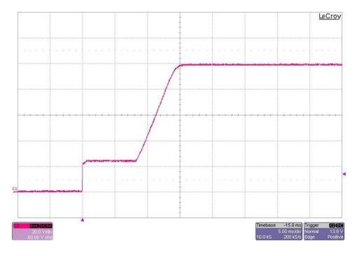
The photo below shows the output voltage startup waveform after the application of 24V in. The 100V output was loaded to 280mA. (20V/DIV, 5mS/DIV)
