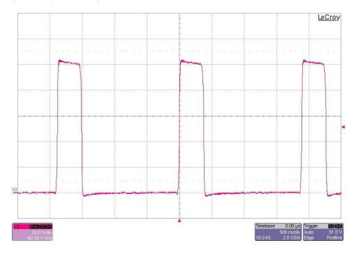
The photo below shows the FET switching voltage. The input voltage is 20V and the output is loaded to 25mA. (20V/DIV, 500nS/DIV)
