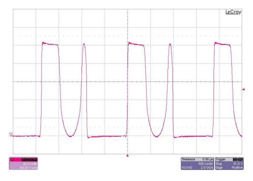
The photo below shows the FET switching voltage. The input voltage is 30V and the output is loaded to 25mA. (20V/DIV, 500nS/DIV)
