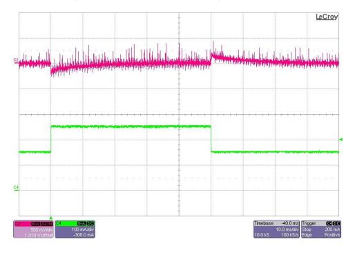
The photo below shows the output voltage (ac coupled) when the load current is stepped between 150mA and 250mA. Vin = 30V. (500mV/DIV, 100mA/DIV, 10mS/DIV)
