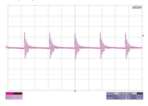
The 100V output ripple voltage is shown in the figure below. The image was taken with the output loaded to 280mA. The input voltage is set to 30V. (200mV/DIV, 1uS/DIV)
