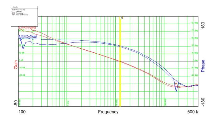
Input voltage = 6.5VPhase margin  $= 62^{\circ}$ Bandwidth = 12 kHz
