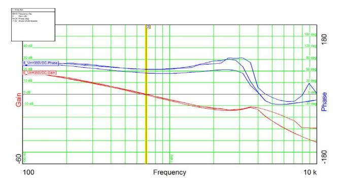
$\begin{array}{ll} \text{Input voltage} & = 140 \text{VDC} \\ \text{Phase margin} & = 56^{\circ} \\ \text{Bandwidth} & = 0.65 \text{ kHz} \end{array}$
