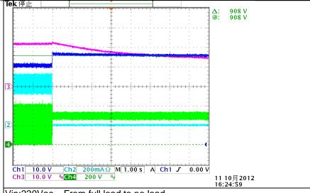
Vin:230Vac From full load to no load
