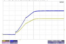
Top, 5V output, 1V/div; Bottom, 3.3V output, 1V/div
