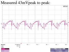
5V Output Ripple (C19), 20mV/div Measured 50mV peak to peak:
