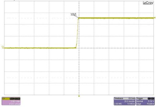
The scope plot below shows the 5V output voltage startup waveform after the application of 48Vdc at J2 (PoE). The output was loaded to 5.0A.
