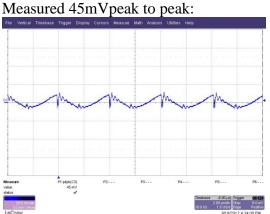
5V Output Ripple (C19), 50mV/div Measured 50mV peak to peak:
