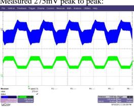
5V Response 50mV/div Measured xxmV peak to peak: (No significant variation higher than switching frequency ripple)
