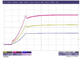
Top, 5V output, 1V/div; Middle, 3.3V output, 1V/div; Bottom, 10V output, 5V/div
