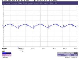
10V Output Ripple (C13), 50mV/div Measured 114mVpeak to peak:
