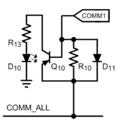
During thermal cycling, the overheat LM3466's fault indicator will blink. After it is latched off, the fault indicator will be lit up steadily
