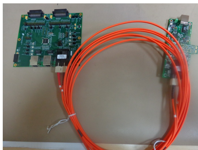
Figure 9. DP83849IVS-EVK Connected with Fiber-Optic Brick
