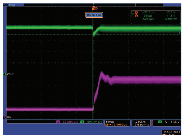
Figure 6. PCMC Transient Response (0% to 80% Load Step)
