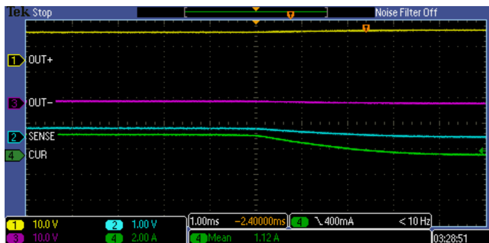
Figure 8: Zoomed-in scope image of forward direction motor stalling
