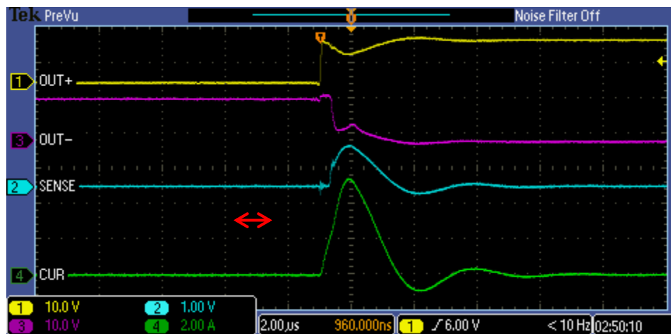
Figure 1: Scope image of motor folding forward from stopped position
