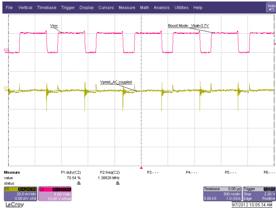
Figure 6. Boost mode Ripple and Duty Cycle; VBAT = 3.7V.
