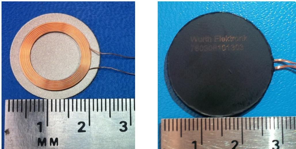
Figure 3. TDK (Left) and Würth (Right) Receiver Coils
