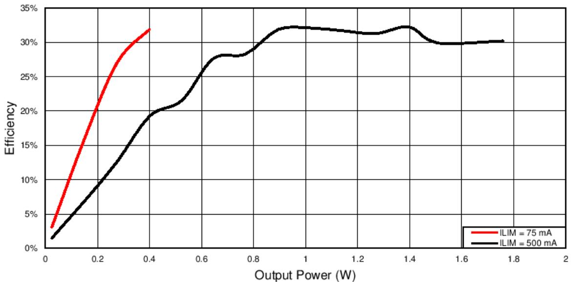
Figure 7 TIDA-00329 Efficiency versus Current Limit Setting (ILIM)
