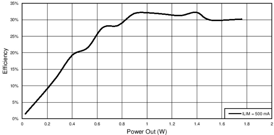
Figure 6 TIDA-00329 Efficiency with bq51003
