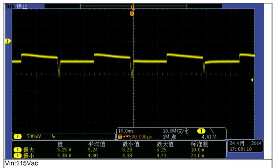
test condition: 0-50% of full load with 10mA pre-load, 0.1A/us, 30ms cycle, 100cm cable
