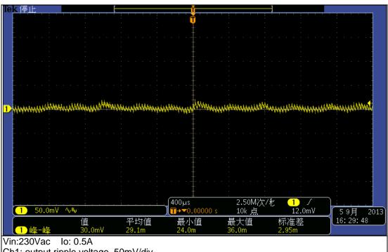
Ch1: output ripple voltage, 50mV/div
