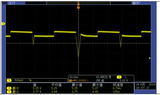
Vin:115Vac test condition: 0-50% of full load, 0.1A/us, 30ms cycle, 100cm cable Ch1: output voltage
