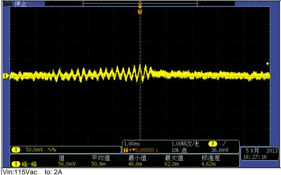
Ch1: output ripple voltage, 50mV/div
