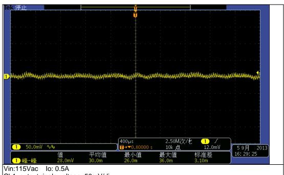
Ch1: output ripple voltage, 50mV/div
