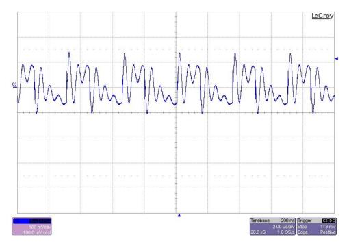
The 28.3V output ripple voltage (AC coupled) is shown in the figure below. The image was taken with the output loaded to 4.5A. The input voltage is set to 28V. (100mV/DIV, 2uS/DIV)
