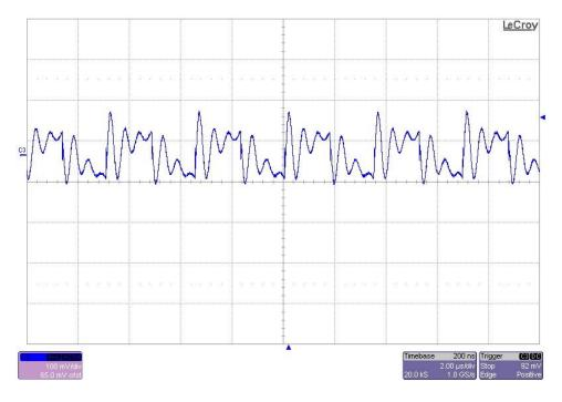
The 28.3V output ripple voltage (AC coupled) is shown in the figure below. The image was taken with the output loaded to 3A. The input voltage is set to 28V. (100mV/DIV, 2uS/DIV)
