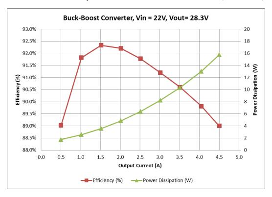
The buck-boost converter efficiency is shown below for Vin = 28V and Vout = 28.3V (Vtrim = 1.25V).
