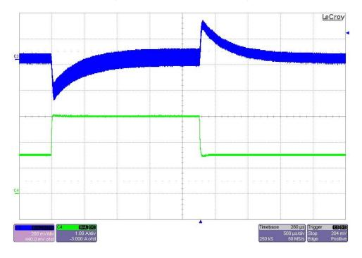
The photo below shows the 28.3V output voltage (ac coupled) when the load current is stepped between 3A and 4.5A. Vin = 28V. (200mV/DIV, 1A/DIV, 500uS/DIV)
