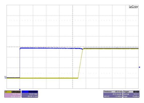
The photo below shows the output voltage startup waveform after the application of 28V in. The 28.3V output was loaded to 4.5A. (10V/DIV, 20mS/DIV)
