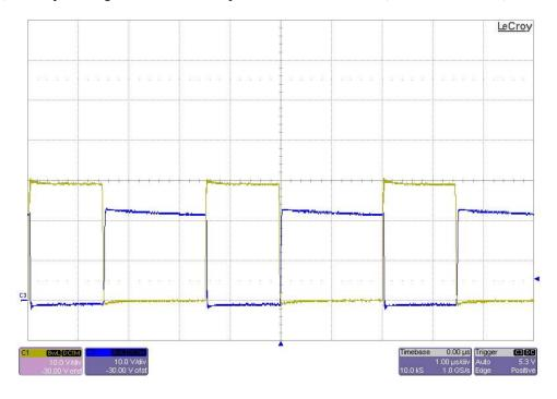
The photo below shows the Q1 FET switching voltage (TP3, blue) and the Q2 FET switching node (TP4, yellow). The input voltage is 28V and the output is loaded to 4.5A. (10V/DIV, 1uS/DIV)
