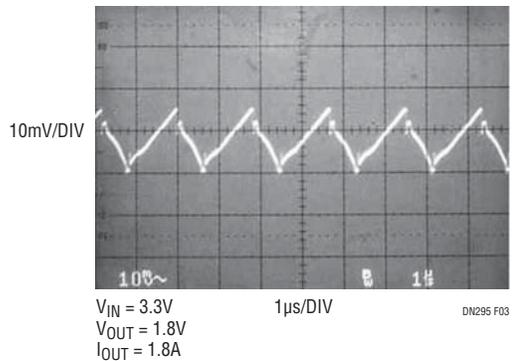
**Figure 3. Output Voltage Ripple for the Circuit in Figure 1**
