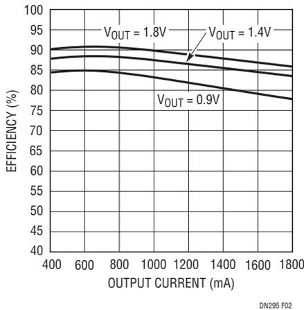
**Figure 2. Efficiencies for the Circuit in Figure 1 where V<sub>IN</sub> = 3.3V**
