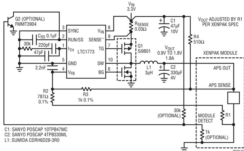
Figure 1. Adaptable Power Supply Using the LTC1773
