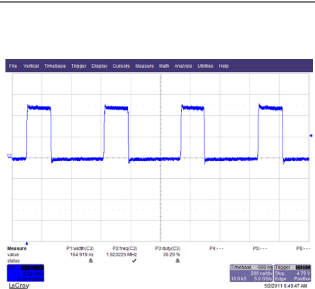
SWN Voltage at 12Vin, 2.2A load CH1=SWN (5V/DIV), 200ns/DIV
