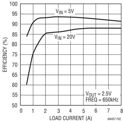
Figure 2. Efficiency vs Load Current of Figure 1
