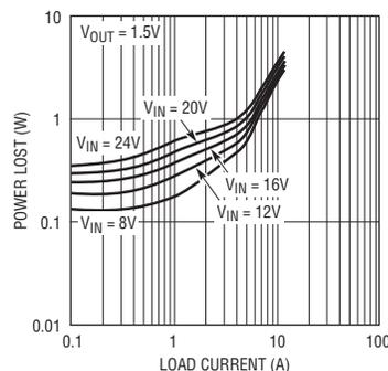
Figure 4. Power Loss Curves for 1-Step Regulator
