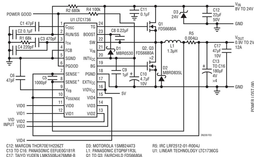
Figure 3. CPU Core Voltage Regulator for 1-Step Application
