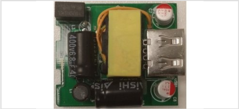
PMP4391: Consumer Electronics, Flyback- Quasi Resonant, Reference Design
