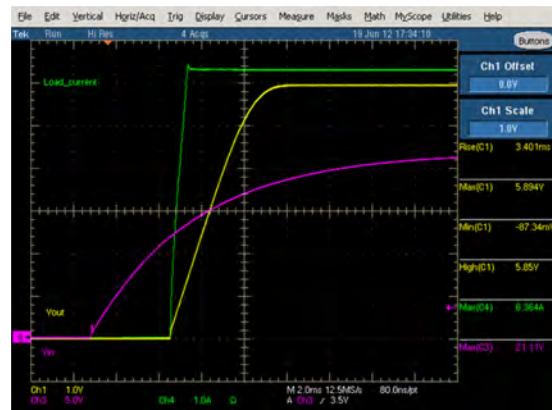
Figure 4. Start-up 22Vin Vo=5.8V, 6A, 5MHz
