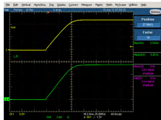
Figure 2. SS Vin=24V, Cref=1nF, CVdr=1μF, Cv3V=1μF, css=68nF, Io=5.5A
