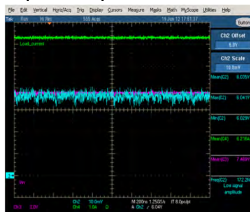
Figure 32. Ripple 8Vin Vo=6V, 6A 5MHz
